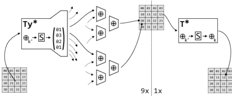
Figure 2: The flow of a byte through the table-network.
