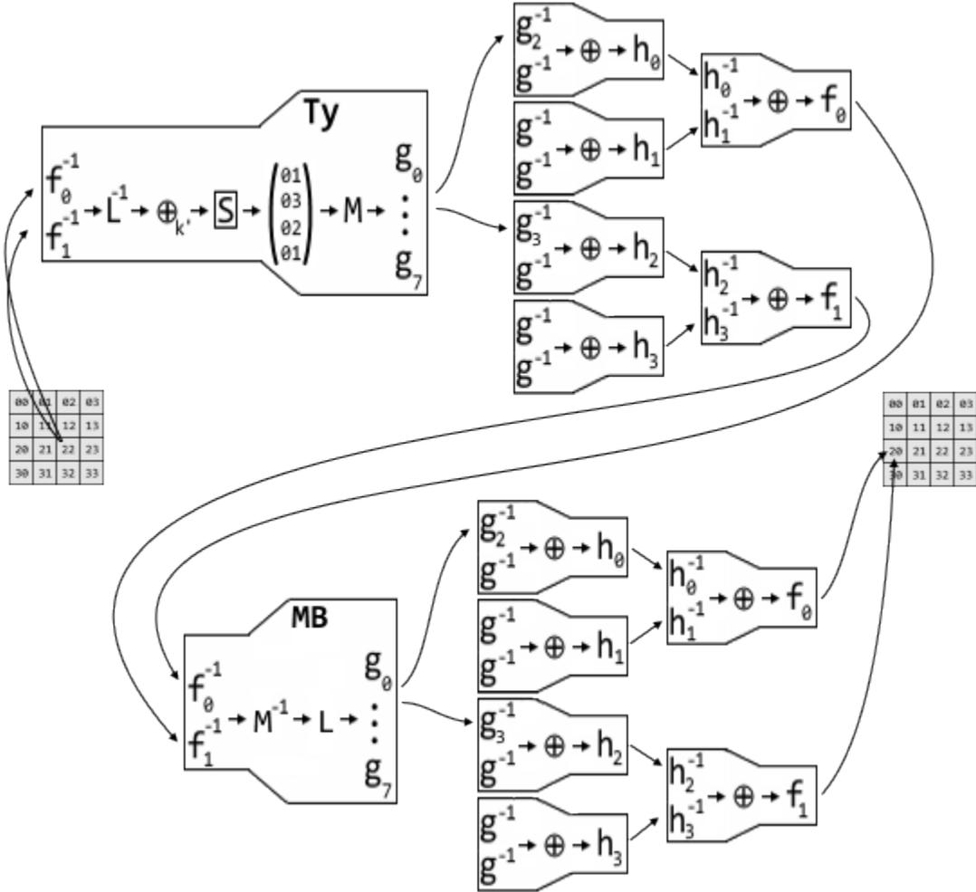
Figure 4: The flow of a byte through the tables from an inner round.
