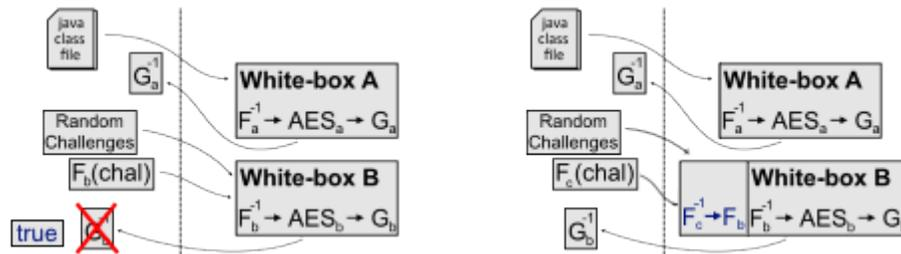
Figure 6: Attack the demo by bypassing the white-box (left) and code lifting (right).
