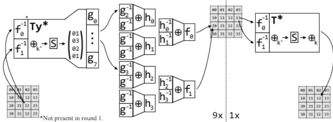
Figure 3: The flow of a byte through the table-network with encodings.
